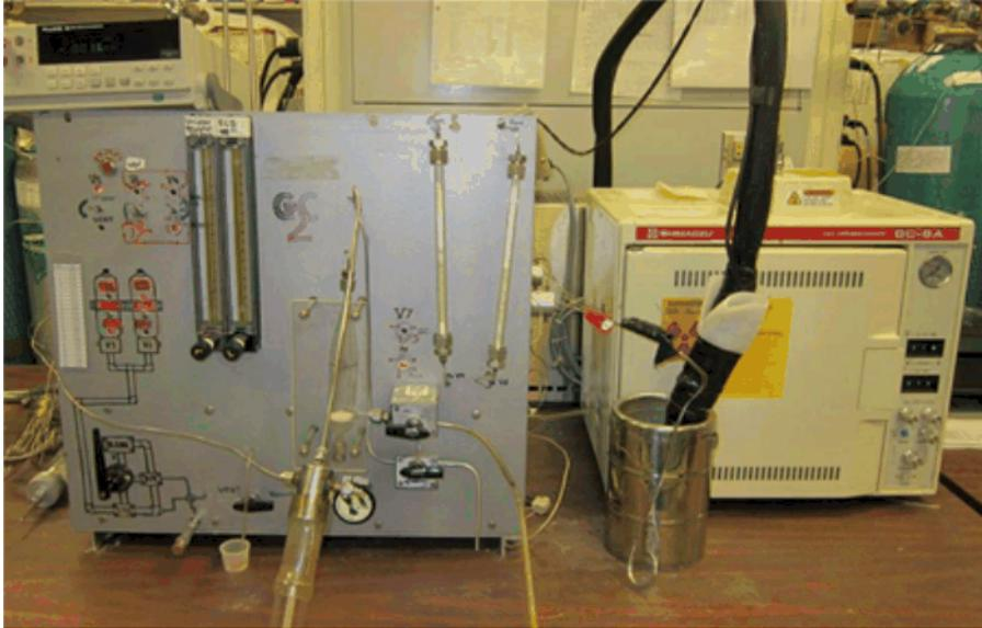
**Fig. 2:** Shimadzu GC-8A [Gas Chromatograph](#) (GC) with an [Electron-Capture Detector](#) (ECD). (Image Source: The Reston Chlorofluorocarbon Laboratory, U.S. Geological Survey) [228, 229].
